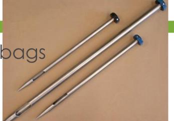
Double Sleeve Trier – used for sampling horizontally and vertically and for a variety of seed size
