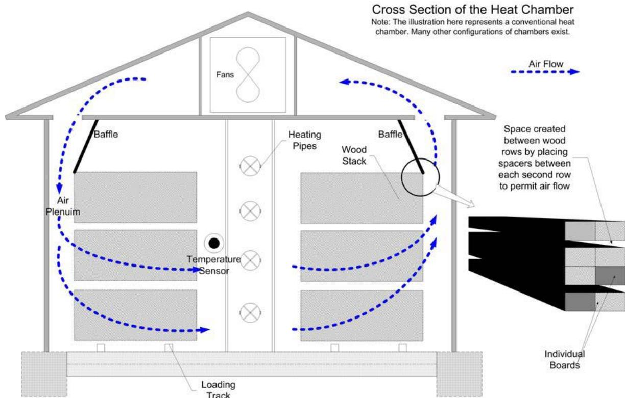
**Figure 2:** A type of heat chamber with the heating pipes in the middle. Temperature sensors should be placed at a location where the air exits the wood stack and is therefore likely to be the coolest.
