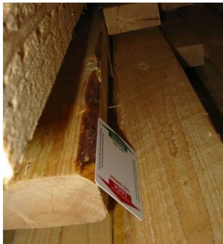
**Image 5** - Bark on the edge is wider than 3 cm and the piece is greater than 50 cm<sup>2</sup>. The bark must be removed or the piece may not be used in wood packaging material.
