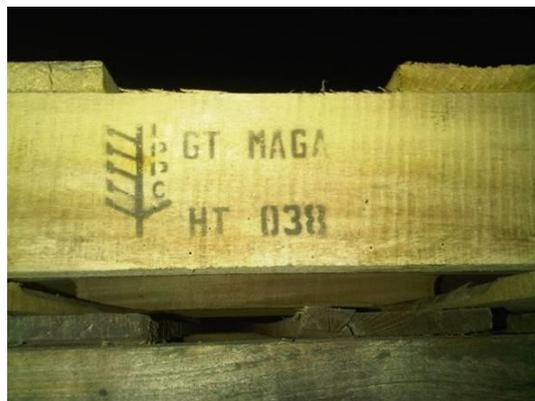
**Image 4<sup>6</sup>** – Mark does not contain the required borders.
