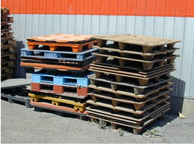
**Image 10** - Plastic and fibre-form pallets
