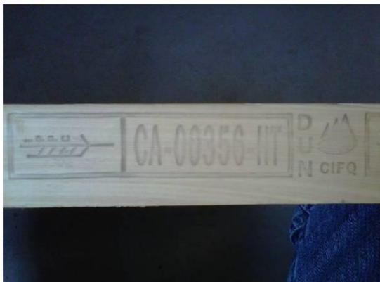
**Image 1<sup>5</sup>** – Mark matches example 6 of Annex 2 of ISPM 15. Additional information included outside the borders of the mark.
