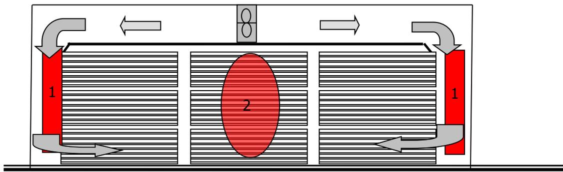
**Figure 4:** A heating chamber in which heating is bi-directional. If the treatment schedule is long, the cold spot may be at the air exit side of the wood (marked 1). Temperature sensors should be placed along the walls of the chamber. If the schedule is shorter, the cold spots are likely to be in center of the wood stack (marked “2”) and sensors should be placed there.
