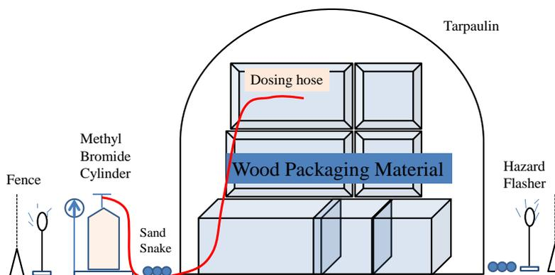
**Figure 5.** Common Layout of Tarpaulin Fumigation
