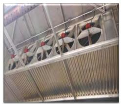
Fans should be used to maximize air flow through the wood stack
