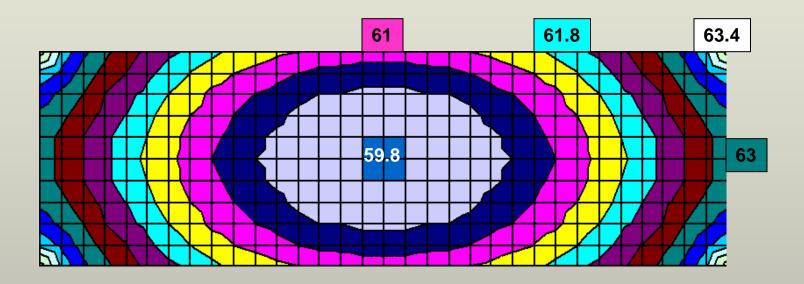
Temperature profile of *Pinus* sawn wood at the end of a 509 minute schedule. Generally this temperature maintained for a further 30+ hr
