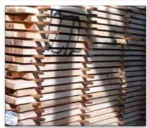
Spacers (stickers) should be used to maximize air flow through the wood
