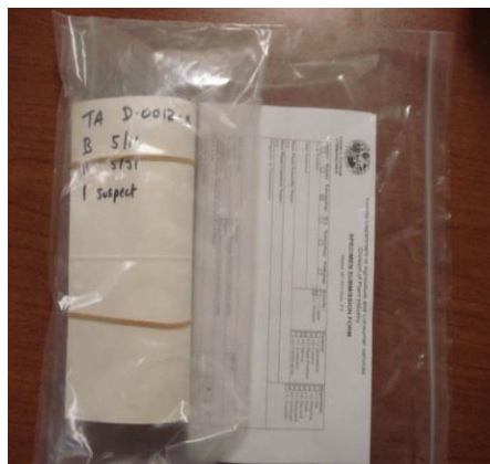
Figure 6. Placement of form and sealed bag with trap into second sealed bag.
